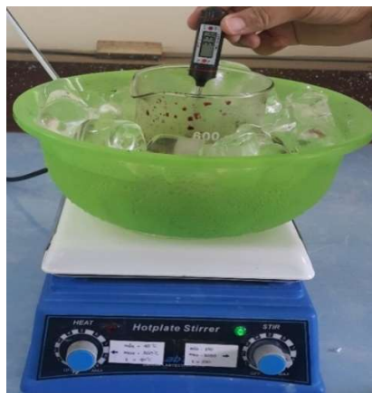
Figure 2. Graphite, \text{NaNO}_3 and \text{H}_3\text{PO}_4 mixture was stirred in ice bath
